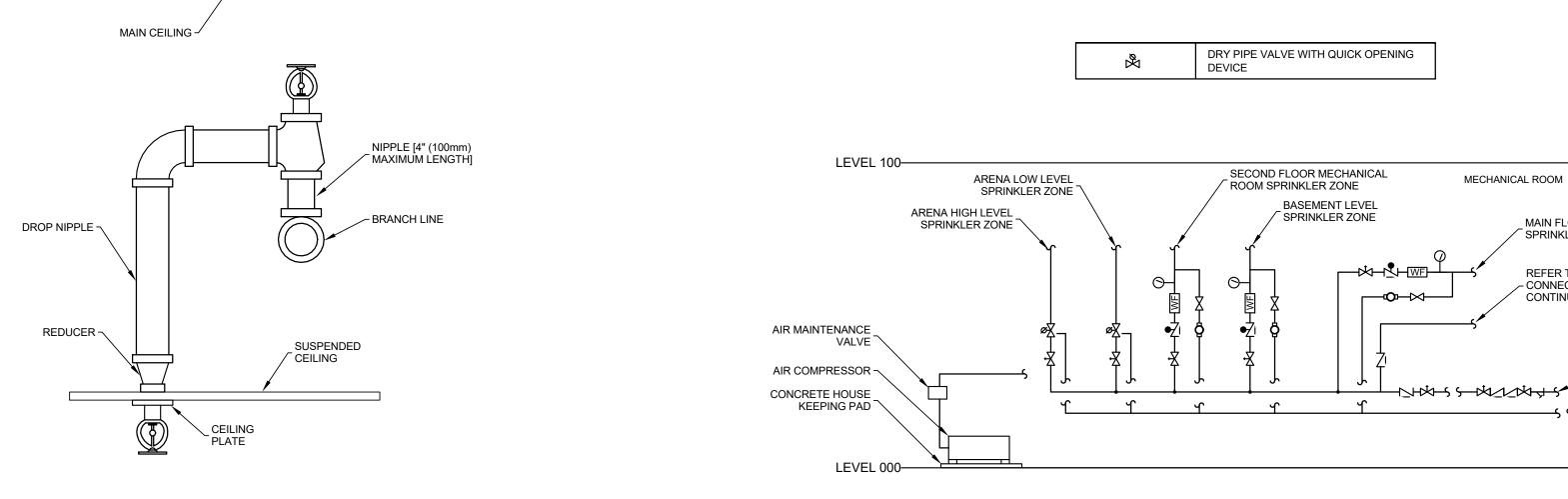
SPRINKLER HEAD BELOW CEILING - REDUCING ELBOW SCALE: N.T.S.
